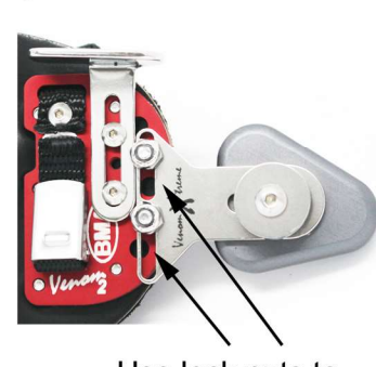
Use lock nuts to lock down plate
